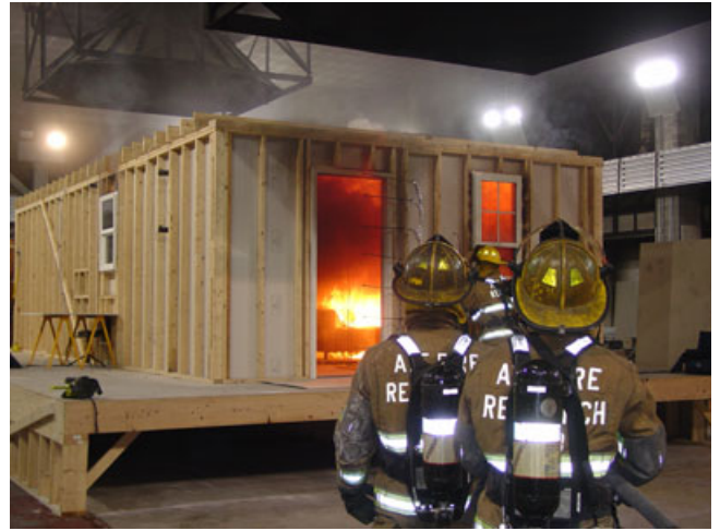
FIG. 4—The structure approaching flashover.
