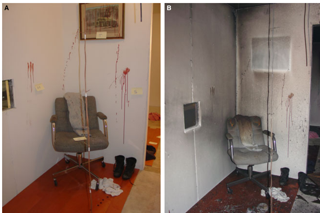
FIG. 7—(A) Dining room before burn. (B) Dining room after burn.
